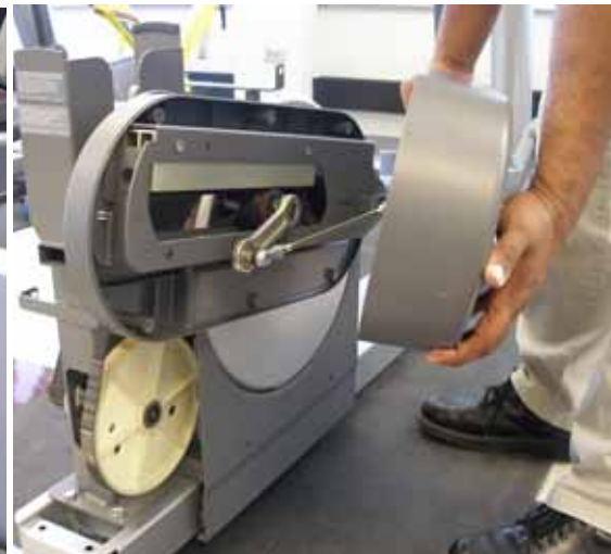
Fig. 4: removing the right outer link cover
